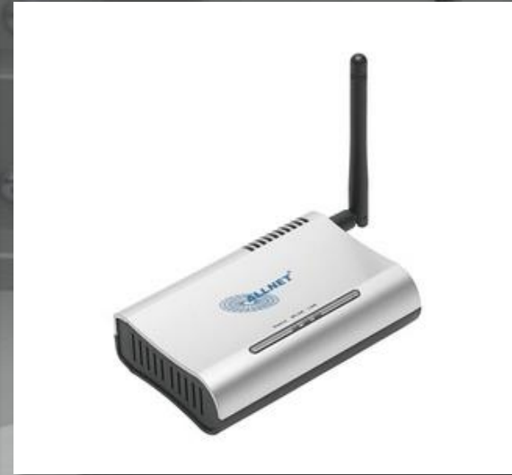
External Access Point
